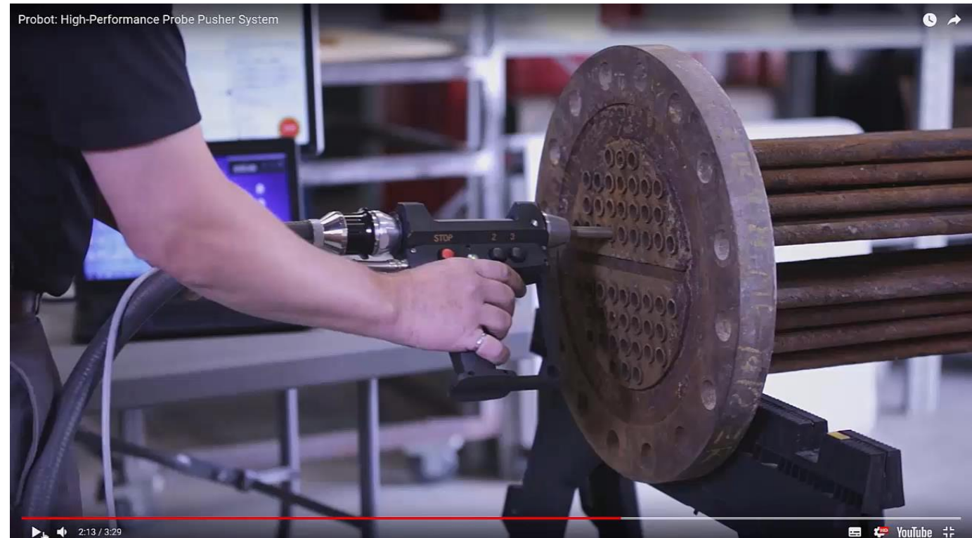
Remote Field inspection using the Probot
